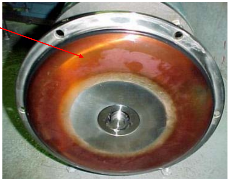
Discoloration effect of rouging
