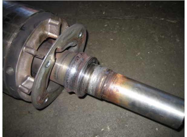
Examples of motor bearing failure
