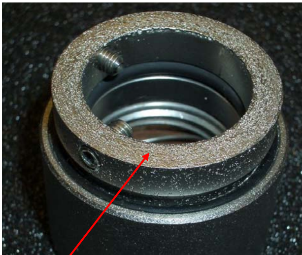
Example of pitting corrosion on stainless steel
