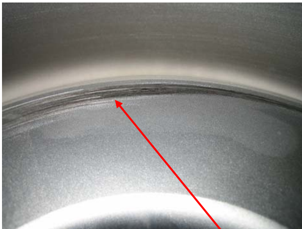
Scoring marks due to ingress of hard foreign object
