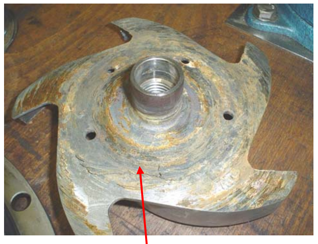
Here the impeller position was adjusted so as not to rub on the pump casing but instead began to rub on the backplate
