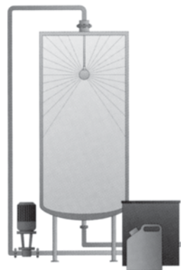
1 Day Others perform "semi-manual" cleaning using static spray balls. This method can take hours
